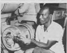
A CASH award of Fls. 30 goes to Antonio Brown of Mechanical-Yard on his selection as Safety Suggester-of-the-Month. He suggested installing guards on lathe motor ends to keep out metal chips. UN PREMIO cash of Fls. 30 to him by Antonio Brown of Mechanical-Yard depends on its selection como Superador-de-Lana pa Seguridad. Ela a sugeri pa instala protection ariba motornan di lathe pa evita chipman di metal.
